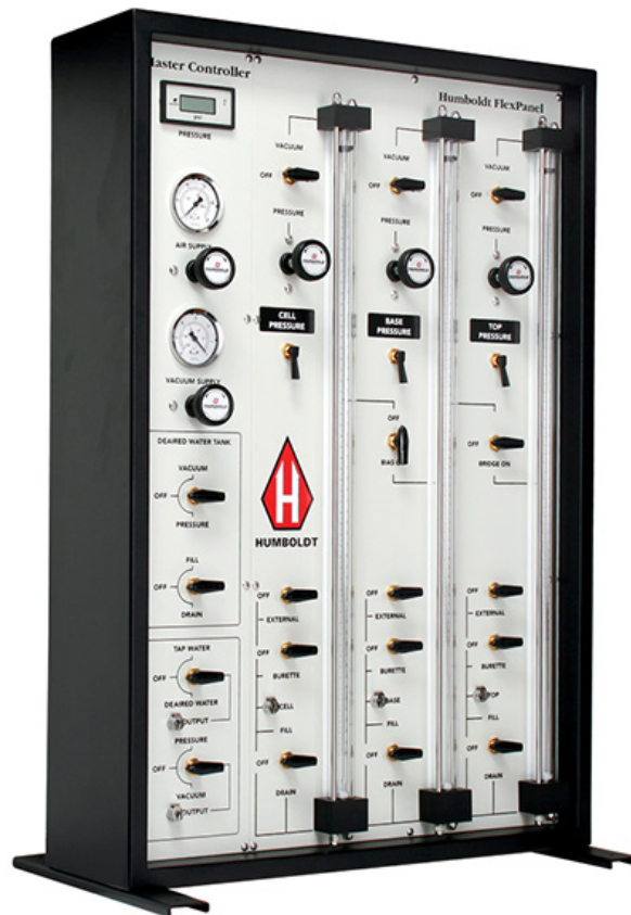
Figure 2.3: Humboldt HM-4150 pressure and vacuum control panel (source: Humboldt Manufacturing).
