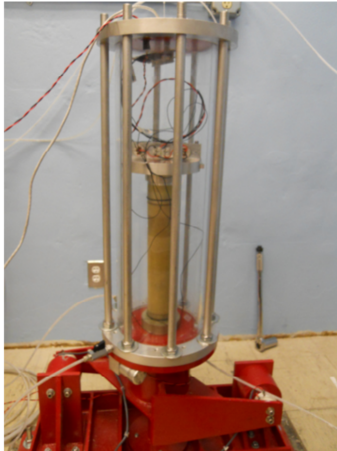
Figure 5.24: 2.8 inch diameter and 11.2 inch height ASTM 20/30 sand specimen.
